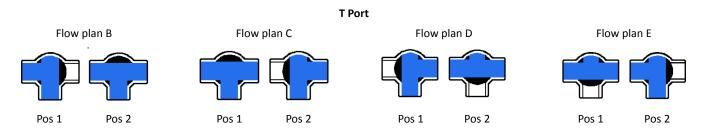
Once you know whether you require an L port or a T port, the next step is to determine the flow plan. The flow going through the valve may come from either direction ie: left to bottom or bottom to left etc. As the actuator will only be turning 90°, decide which flow plan will accomplish your end needs. The positions 1 & 2 of a given flow plan may be reversed to obtain the desired results.
